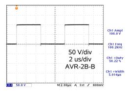
The AVR-1, -2, -3, and -4 models are high-voltage pulse generators capable of driving  $50\Omega$  (or higher) loads and operating over a wide pulse width range. The instruments include IEEE-488.2 GPIB, RS-232, and Ethernet interfaces. For diode loads, these models can be used to provide up to 1, 2, 4, 5, 6 or 8 Amps of pulsed current, if the diode is connected in series with  $50\Omega$ . These models operate over a wide pulse width range - typically 100 ns to 100 us.
